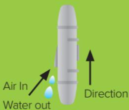
Siphon break must be higher than the water level in the reservoir.
